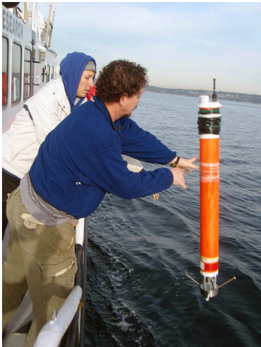
Figure 1: Deployment of a seafloor pressure instrument from a research vessel in Puget Sound. This version contains a Paroscientific model 6000-200A pressure transducer which has been optimized for maximum resolution. Visible at the top is a power plug. Inside the top end cap is an acoustic transducer. A unique coded sequence sent to this transducer triggers a logic sequence that burns a wire, releasing the weight at bottom and allowing the instrument to surface with the bottom end pointed upward. A GPS antenna in the end cap receives position and time, which are broadcast as a 900 Mhz digital radio signal through a separate antenna. The radio signal and flasher aid in shipboard recovery.
